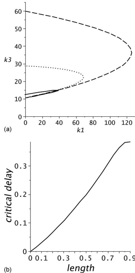
FIG. 2. Stability of the upright fixed point for the model (3) with parameters corresponding to the experimental setup in Ref. 13 and  $k_2$  and  $k_4$  chosen according to Eq. (13). (a) The stability region is terms of  $k_1$  and  $k_3$  for  $\tau = 0.01$  (dashed),  $\tau = 0.05$  (dotted), and  $\tau = 0.1$  (solid). (b) Effect of changing the length  $\ell$  on the critical delay  $\tau_c$ .
