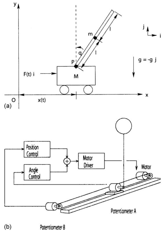
FIG. 1. (a) Schematic representation of an inverted pendulum stabilized by the movements of a cart.  $M$  is the mass of the cart and  $P$  is the pivot point of the pendulum. See text for definition of other parameters. (b) Implementation of delayed feedback control of an inverted pendulum that utilizes the carriage mechanism of a dc-motor-operated plotter (Ref. 14) (see Sec. IV for details).
